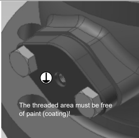
Fig. 5-1: Ground connection Valve Type 72, 73, 82
