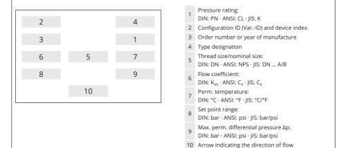
Fig. 2-4: Nameplate of Type 2441 Input Pressure Regulator
