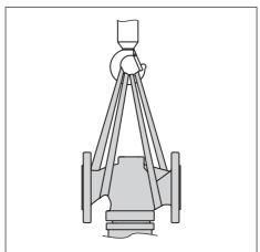
**Fig. 4-1:** Schematic drawing of lifting points on the regulator
