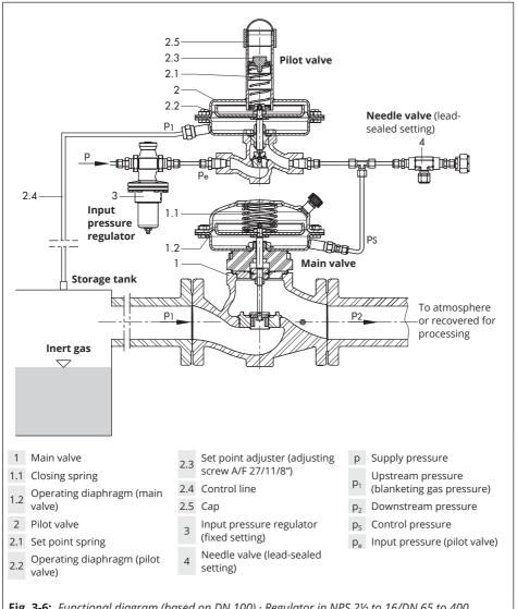
Fig. 3-6: Functional diagram (based on DN 100) · Regulator in NPS 2½ to 16/DN 65 to 400
