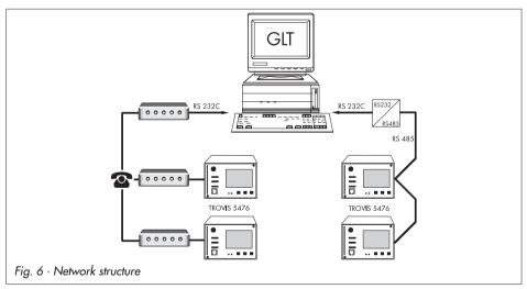
The TROVIS 5476 Controller is fitted with either a RS-485 port or a RS-232-C port depending on the order. The optional operation between both versions or a conversion to a different port version is not possible.
