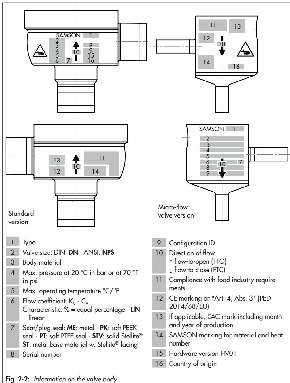
**Fig. 2-2:** Information on the valve body
