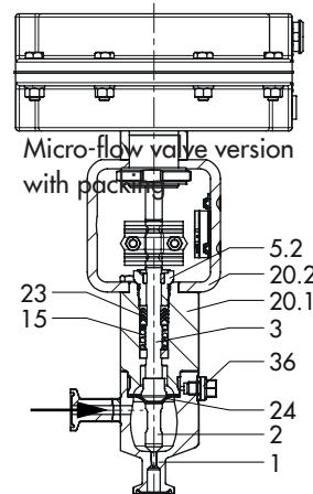
**Fig. 9-2:** Type 3349 Valve with Type 3271 Pneumatic Actuator
