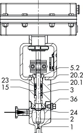
Fig. 3-1: Type 3349 Valve with Type 3271 Pneumatic Actuator
