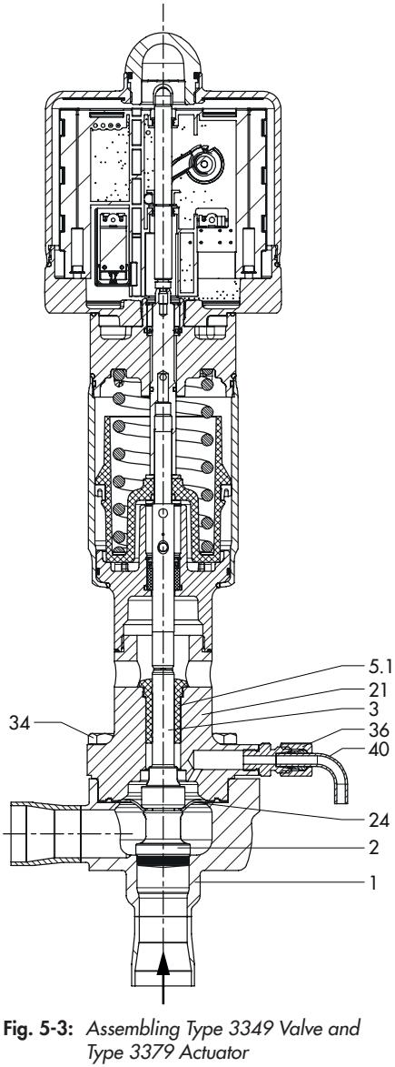
Fig. 5-3: Assembling Type 3349 Valve and Type 3379 Actuator
