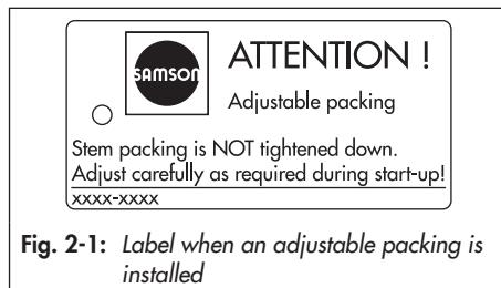
**Fig. 2-1:** Label when an adjustable packing is installed
