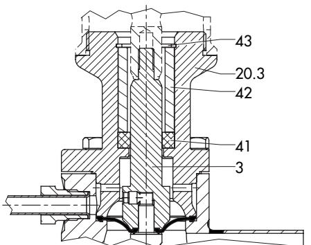
Fig. 9-6: Stem seal (micro-flow valve version without packing)
