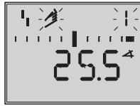
Code 1 Position valve using the rotary pushbutton, the current angle of rotation is indicated
