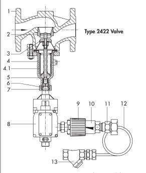
Type 2401-2 Pressure Element with limit adjustment, screw fitting, capillary tube and strainer
