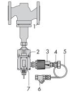
Fig. 3: PL/SPL with globe valve (Type 2111/Type 2422) and electric signal transmitter
