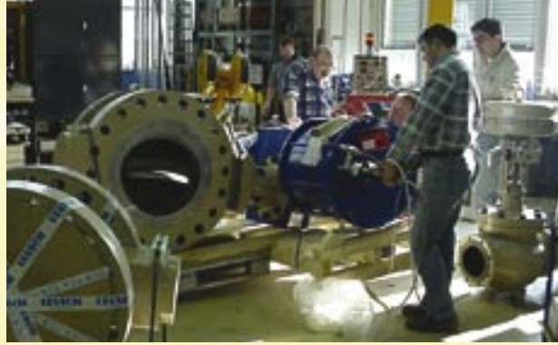
Assembly of the LEUSCH butterfly valves in the Sultanate of Oman. · All the products manufactured by LEUSCH have a high technical standard and have been extensively tested at all manufacturing levels. Like SAMSON, LEUSCH is certified according to ISO 9001:2000.
